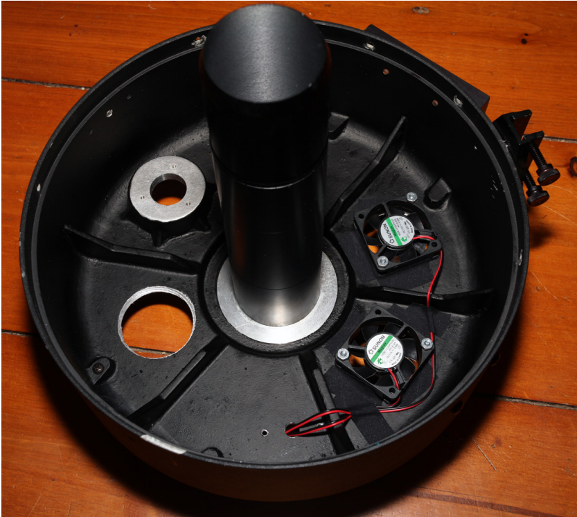
Figure 2. View of the mirror cell with two fans installed and single 2" exhaust port.
