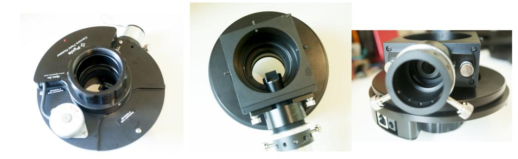
Pyxis SCT connection has interior lip that mates with flange approximately 9mm inside. OAG guide port is narrower deep inside, so guide camera cannot slide in very deeply. OAG is used in reverse orientation from normal, for better connectivity on each side. Pyxis connects directly to SCT port instead of the standard 2" adapter.
