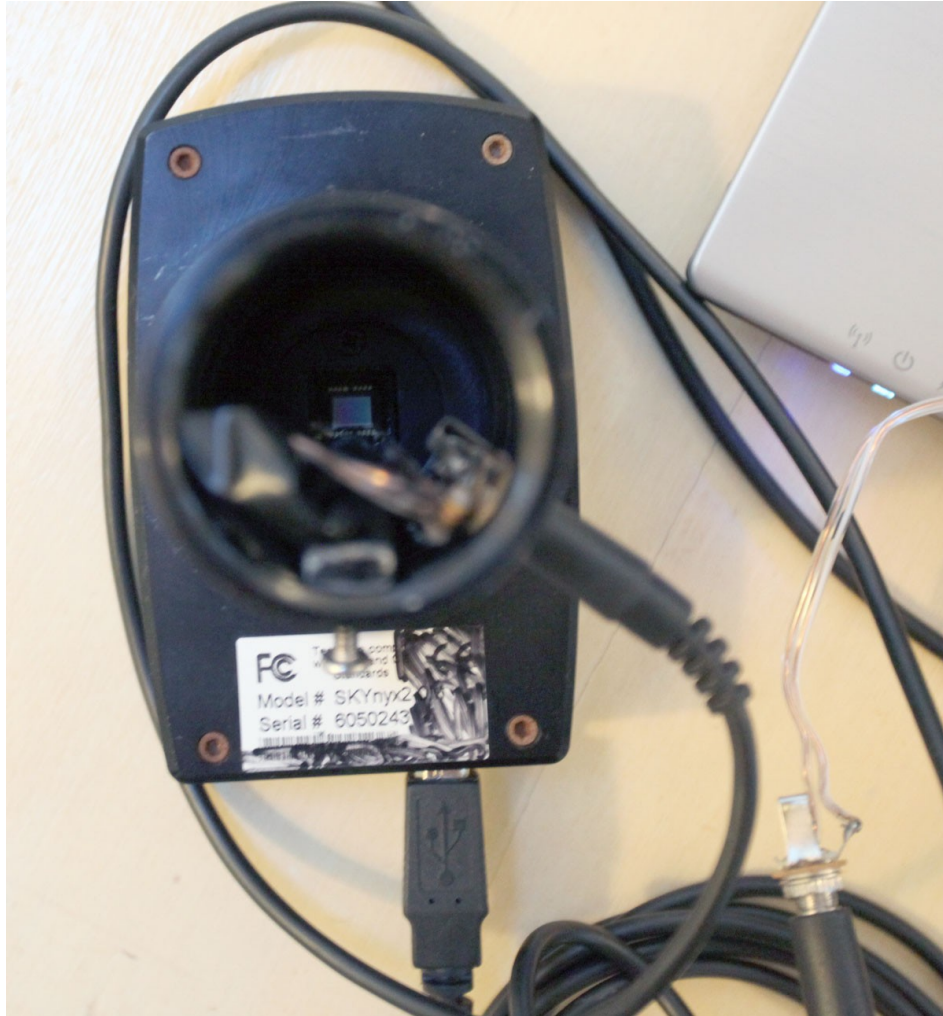
Figure 4b. View into the Lumenera camera showing the LED time spot projection device.
