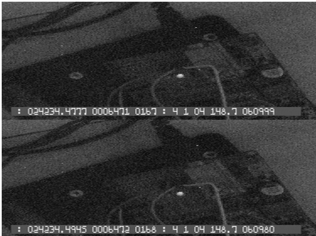
Figure 12. The same view as Figure 11, but using LiMovie's “field” display to show the two separate 16.8ms fields contained in the frame. Note that the OSD text is clearly visible in each field, and each field has its duration values shown: 16.7 ms above, and 16.8ms below. The dark background of the text helps with character decoding by software, and the colons serve as markers to establish the text size and location.
